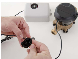
Figure 15: Gray Wires in Slot
